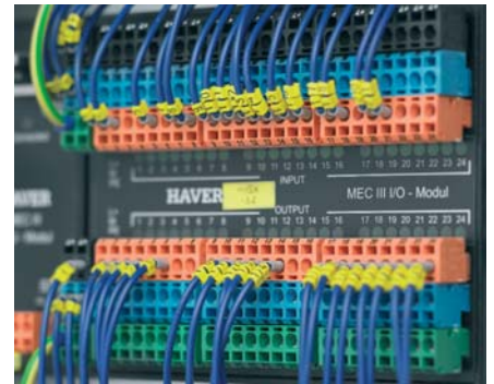
I/O module developed for specific customer needs with PCB plug-in connectors using tension clamp technology.
