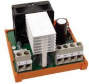
RSD-40A 20A per Input or 40A Input per Unit Diode Module with Status Indication
